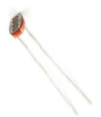
The Photocell is a light sensor in which the resistance varies according to the intensity of light. The resistance reduces when it is in brighter surroundings. We have to set up a threshold value for the measurements of the intensity because it cannot give the precise measurements. If the measurements are below the threshold then it is dark, else it is bright.
